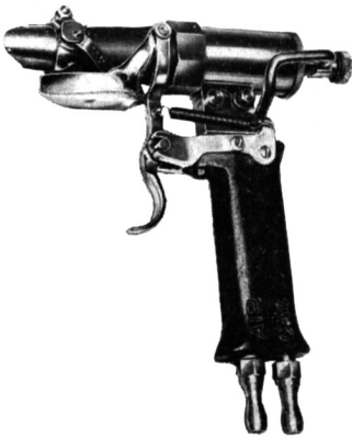
Figure 238. a BUSMC Pneumatic Treeing Machine with hot blast tool. b Close-up of hot blast tool.
