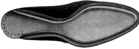
Figure 205. Sewn and stitched veldtschoen. The forepart is stitched in the channel and the waists Blake-sewn up to the joint, also in a channel.
