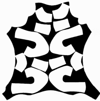
Figure 66. Goatskin with three-quarter court shoe and heel cover lay-out.
