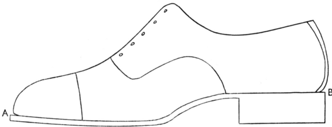
Figure 219. Range of shoe. There must be continuity of line from A to B.
