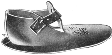
Figure 194. Veldt upper after seat flanging.
